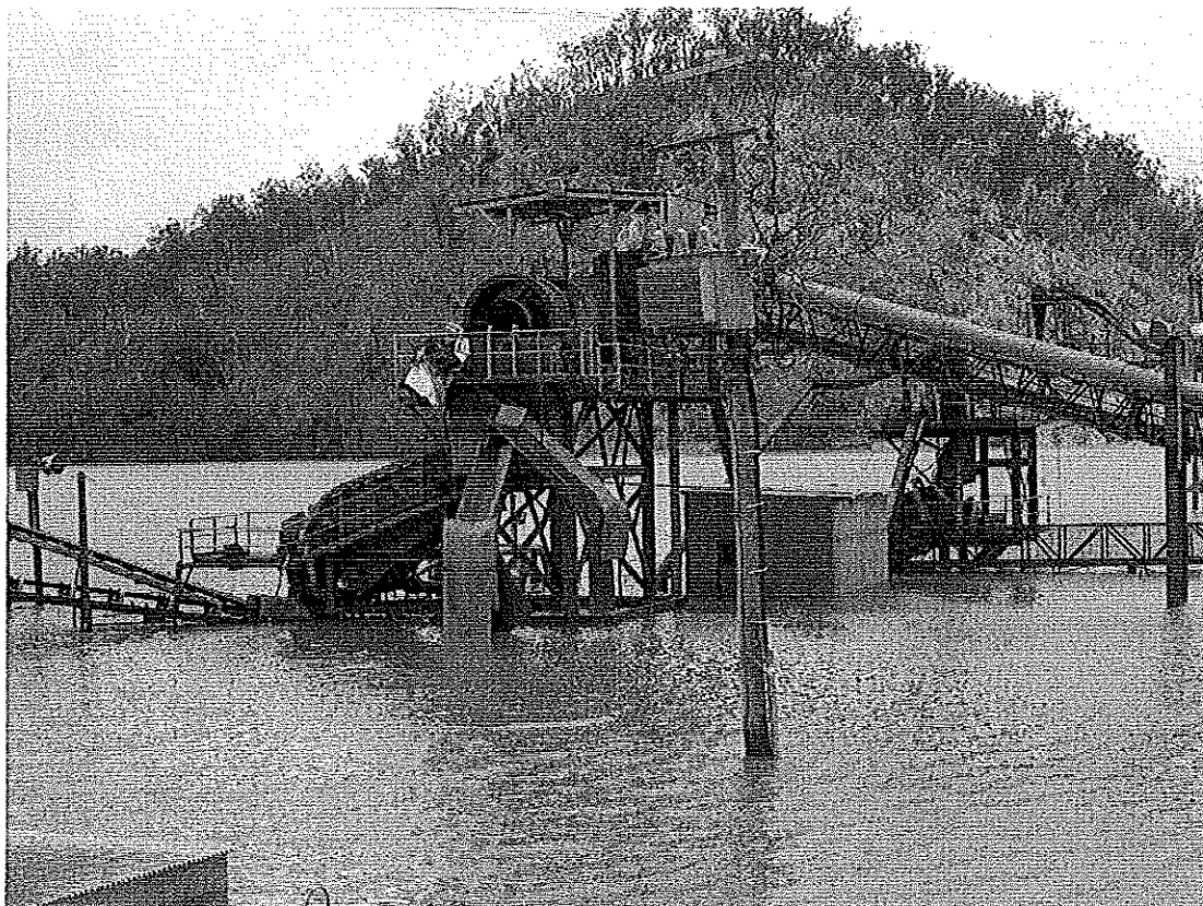
Substantial damage to fixed sand plant and concrete plant.
