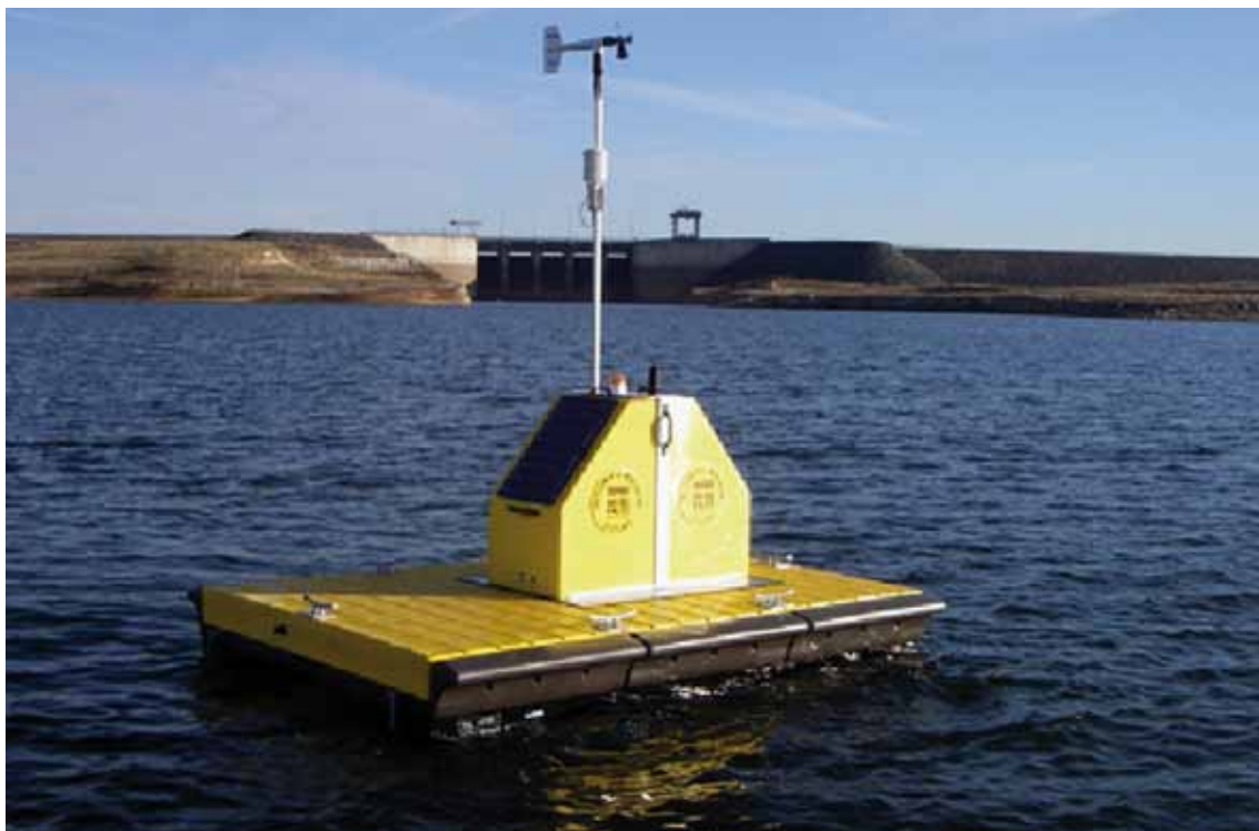
Figure 13 One of Seqwater's telemetered water quality profiler and meteorological stations on Lake Wivenhoe.
