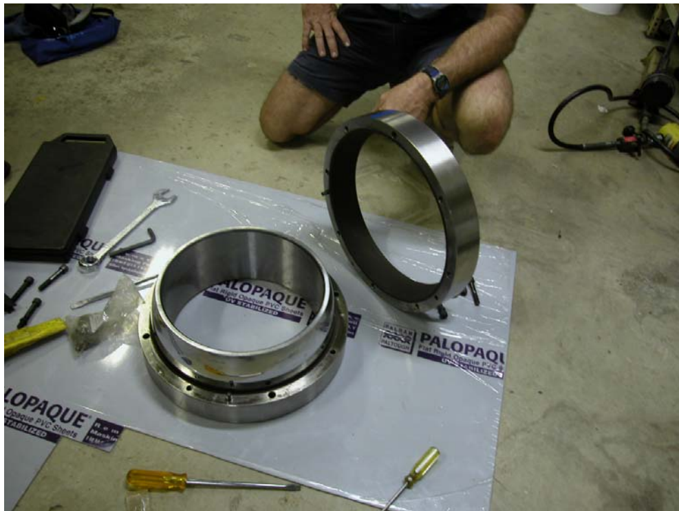
Photo 2 Wivenhoe Dam: Spare Bush, Dismantled Note Black PTFE coating on outer ring
