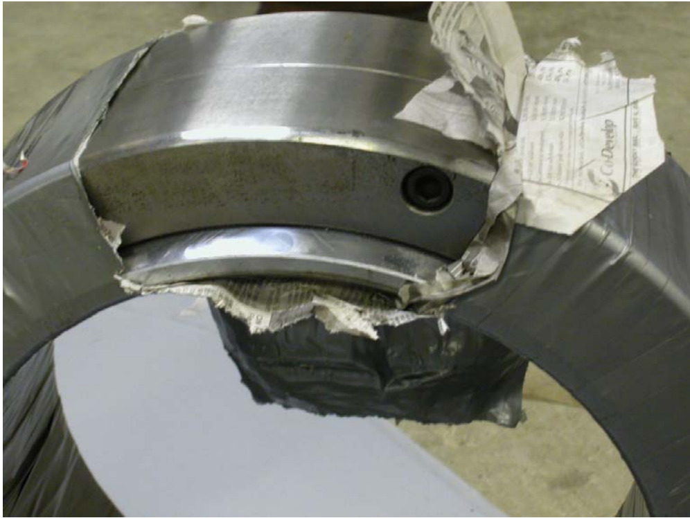
Photo 1 Wivenhoe Dam: Spare Bush, Assembled Note protruding chromed surface of inner ring
