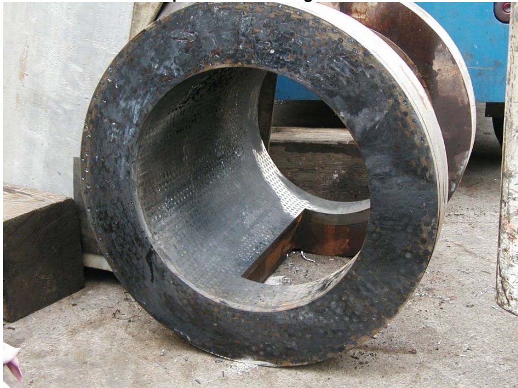
Photo 6 Priest Rapids Dam Washington State USA Deteriorated Lubrite Bush Replaced by ORKOT
