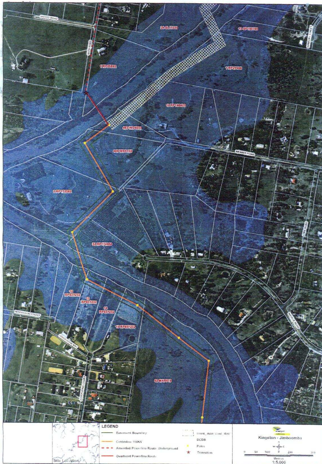
Figure 3 – Energex map showing the proposed powerline at crossings 1 and 2, the Q100 flood level and the proposed 4 concrete power poles in line with the Natalie Road cliff, which is a known high flood current section of the river.
