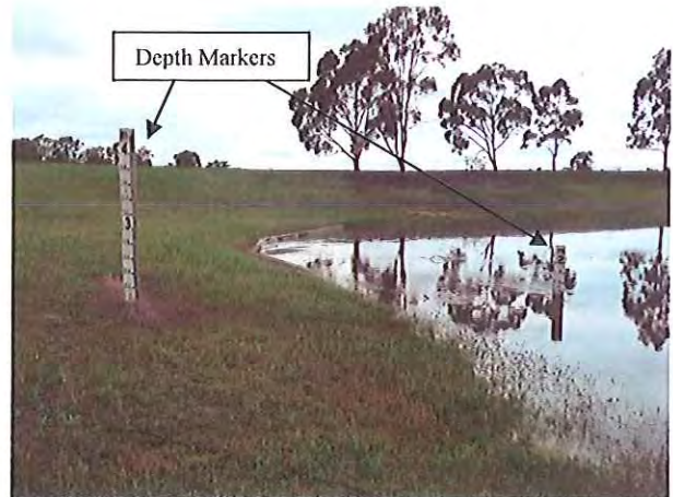
Note the two Water Depth Markers. The Right Marker measures 0-2 meter deep water. (now reading 1.5 meters deep)
