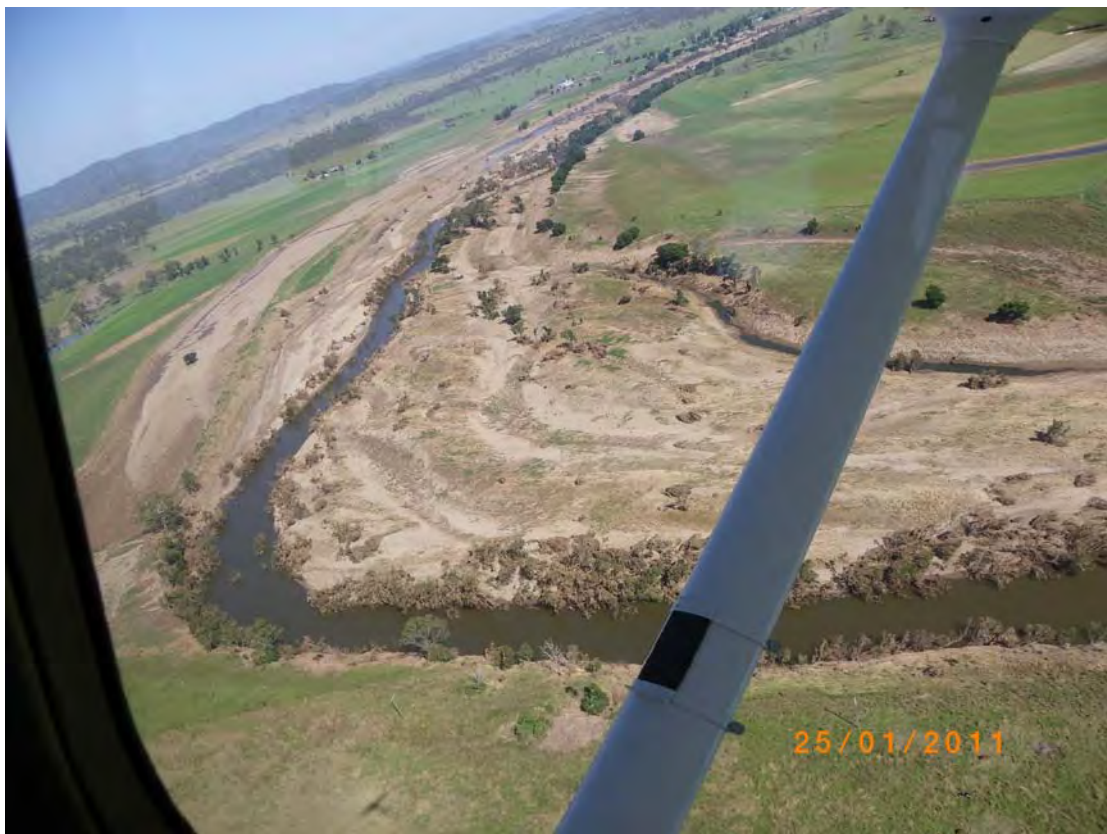
Figure 16 Aerial view of riparian erosion in Upper Brisbane Catchment
